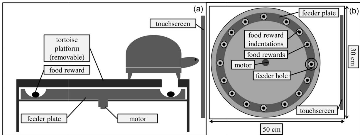
Fig. 1. Tortoise touchscreen apparatus: (a) side view of the Skinner box, (b) top view of the feeder plate (illustrations not drawn to scale).
